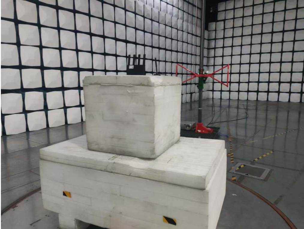
Radiated Emissions Above 1GHz View
